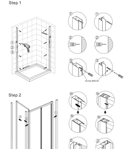
Ensure wall profiles are plumb. Adjust enclosure to be square and level. Wall post and profile should be adjust to square the doors and Ensure open door smooth.
