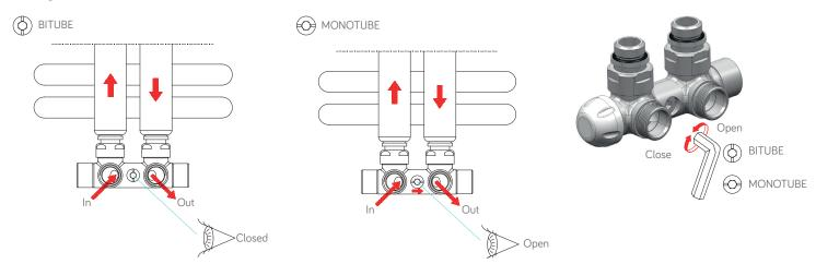
In order to change configuration of the valve from monotube to bitube close the by-pass using 6 mm Allen key rotating it in vertical direction as shown in the picture. Open the by-pass in order to make monotube configuration.
